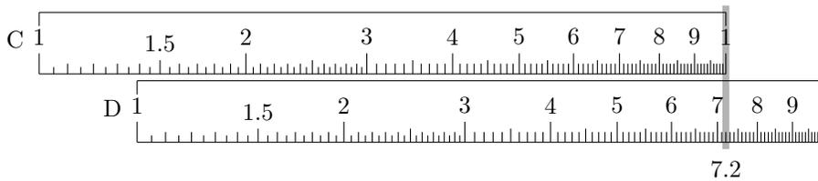
Now find the smaller number, 5.5, on the C scale, and read the D scale under it:
